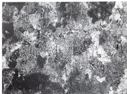
Figure 2.36. An interference-microscopic photograph of a iridium surface after one hour of catalyzing the CPO process at 1000 °C. The different color densities indicate differences in height of about 1 \mu\text{m} [115] .
