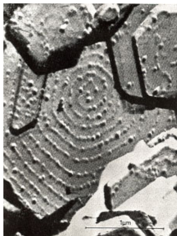
Figure 2.27. Electron micrograph of a hexagonal crystal of \alpha\text{-TiCl}_3 . The dots are believed to represent polypropylene chains growing on sites located along a crystal growth spiral [93] . Stereoregular polymerization occurs by selective self control of the growing polymer chain that leads to preferred alkene insertion [92] . This is very similar behavior to that found in the corresponding homogeneous single-site cyclopentadienyl-Ti or -Zr catalysts. The \text{TiCl}_3 edge sites can be considered the inorganic surface analogues of homogeneous organometallic complexes and display very similar chemistry. Improved heterogeneous catalysts have been designed using selected basic coadsorbates to optimize stereoregularity.
